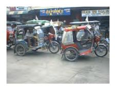
Tricycles are motorcycles attached to or covered within a steel cab. These are common and inexpensive transports typically for distances of a few kilometers.
